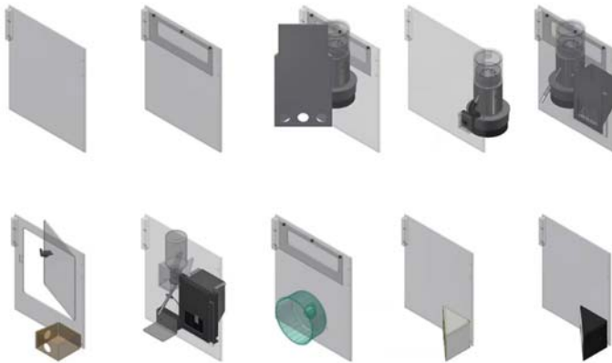
Figure 2 Examples of the components of the PhenoTyper cage.
